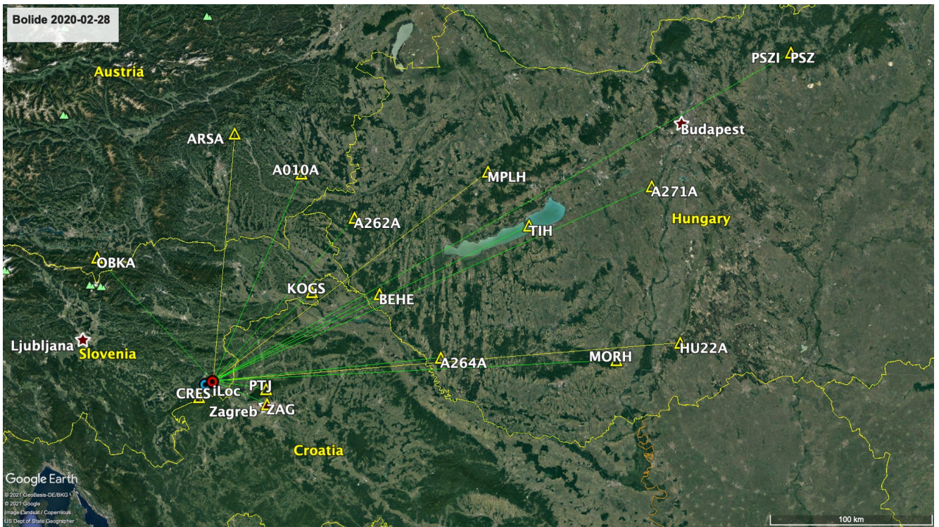
Figure 13. Seismo-acoustic location (red circle) of the bolide over Croatia and Slovenia. The PSZI infrasound array and the seismic stations are shown as yellow triangles.
